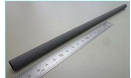
Φ10mm × 280mmL Cladding Tube ( \text{SiC}_f\text{-SiC} )
