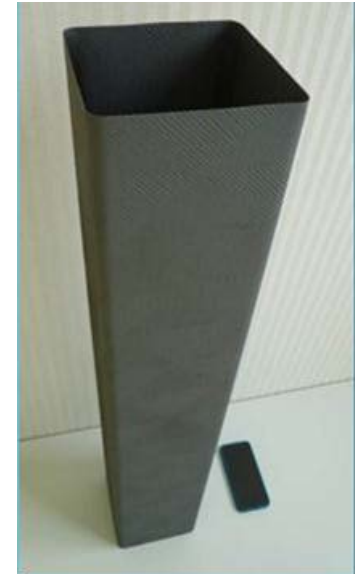
132.5mm × 800mmL Channel Box ( \text{SiC}_f\text{-SiC} )
